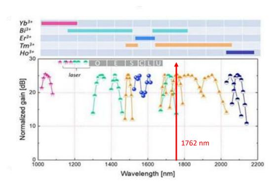
Graphical summary of the infrared wavelength bands covered by single clad doped fiber amplifiers in 2024.
